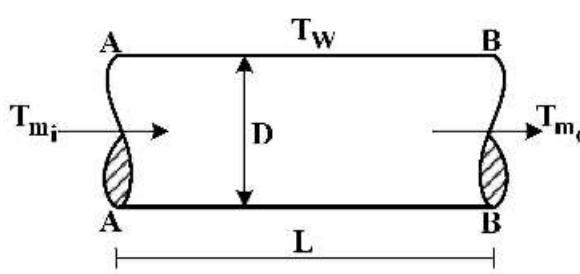
$$T_{m_0} = T_w \left[ 1 - \exp\left(\frac{-\bar{h}L}{\rho C_p D u_m}\right) \right] \quad (1)$$
