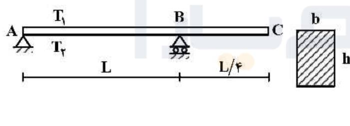
$$\frac{5}{32} \alpha L^3 (T_2 - T_1) \downarrow \quad (1)$$
