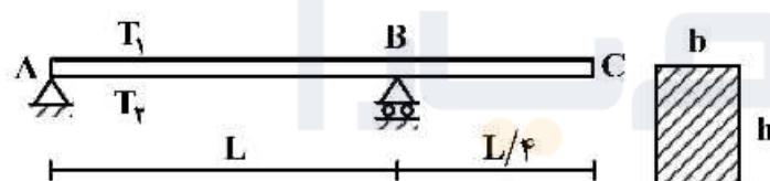
$$\frac{5}{32}h\alpha L^3(T_2 - T_1) \downarrow \quad (1)$$
