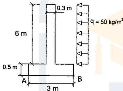
(۱)  $\sigma_B = 2378 \text{ kg/m}^2$  و  $\sigma_A = 2682 \text{ kg/m}^2$
